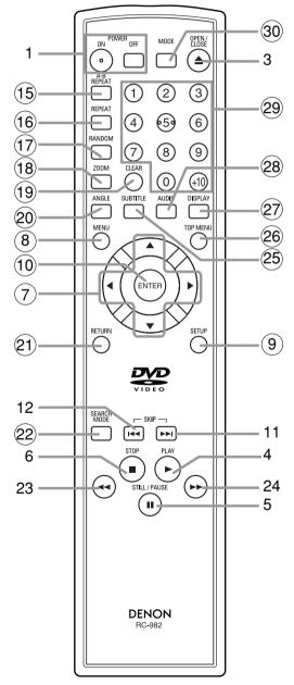
The buttons with circled numbers can only be operated with the remote control.
