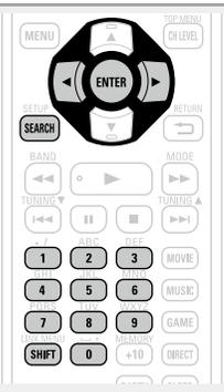
**3** Place the cursor at the character to be changed with  $\triangleleft \triangleright$  and press the number button (**0 – 9**) until the desired character is displayed.
