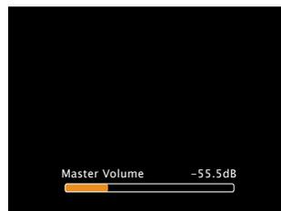
Status display: The operating status appears briefly on the screen when the input source is switched or the volume is changed.
