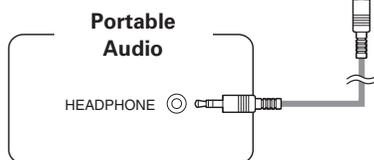
Connect this unit and portable audio player using a separately sold mini-stereo audio cable.
