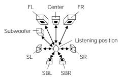
**1** Press the CURSOR  $\triangleleft$  or  $\triangleright$  button to set the distance from the front L speaker to the listening position, then press the ENTER or CURSOR  $\triangledown$  button to switch to the front R speaker setting.
