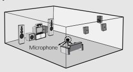
\* Place the microphone on a tripod or level surface.
