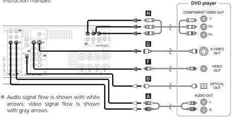
• For best picture quality (especially with progressive DVD and other high definition sources), choose the component video connection to your monitor TV. S-Video and composite video outputs are also provided if your TV does not have component video inputs.
