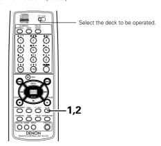
During playback, press the repeat A–B button at the position at which you want to start repeating (point A).
