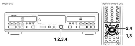
Set the unit to the setup mode, then turn the jog dial of the main unit or press the automatic search button of the remote control to display "A.T. Mark?".
