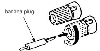
Turn clockwise to tighten, then insert the banana plug.
