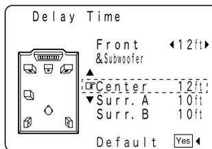
Example: When the distance is set to 12 feet for the center speaker (L1)
