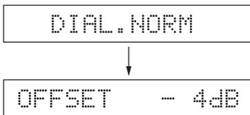
The number indicates the normalization level when the currently playing program is normalized to the standard level.
