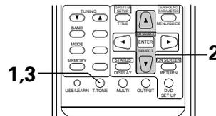
3 After completing the adjustment, press the T. tone button again.
