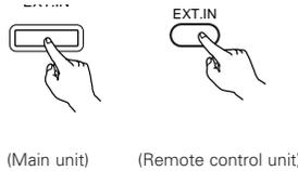
Once this is selected, the input signals connected to the FL (front left), FR (front right), C (center), SL (surround left) and SR (surround right) channels of the EXT. IN jacks are output directly to the front (left and right), center and surround (left and right) speaker systems as well as the pre-out jacks without passing through the surround circuitry.
