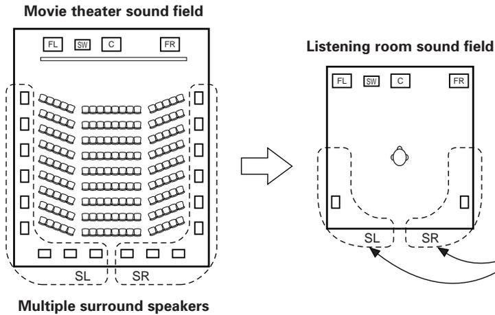
In this case it is important to achieve the same sense of expansion as in a movie theater with the surround channels. To do so, in some cases the number of surround speakers is increased (to four or eight) or speakers with bipolar or dipolar properties are used.
